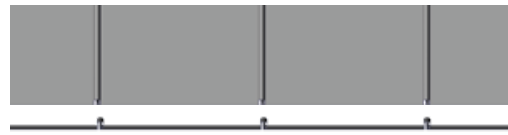
Standing Seam Metal Roof
